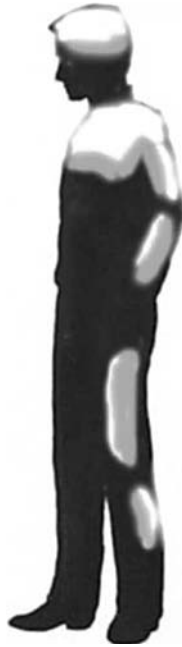
FIGURE 6.5 Representation of the millimeter-wave illumination of a human in an outdoor situation with cold temperature shown bright and warm dark.
