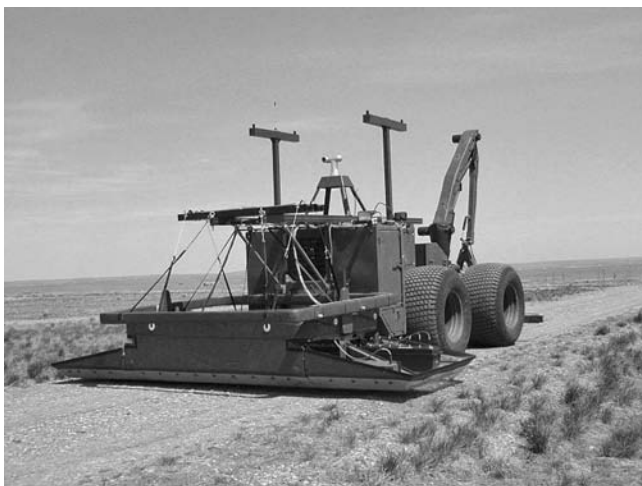
FIGURE 7.13 Photograph of downward look 32-channel array system used on MINDER system (with kind permission ©ERA Technology).
