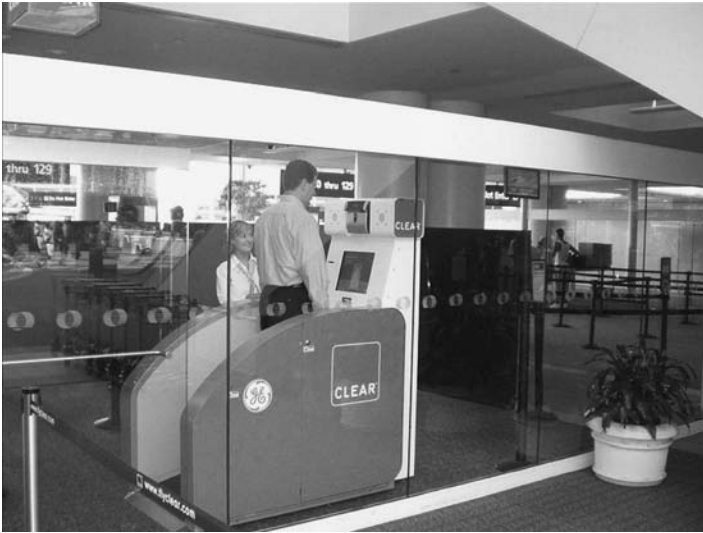
FIGURE 4.24 Integrated shoe detector developed by GE Security (with kind permission ©GE Security and SPIE © 2007).
