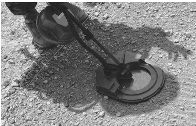
FIGURE 4.27 U.S. Marines AMD NQR technical demonstrator coil (with kind permission ©GE Security).
