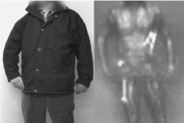
FIGURE 7.23 Images from a 94-GHz passive scanning system (with kind permission Smiths Detection, Ireland).
