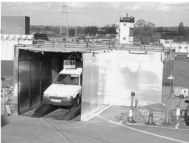
FIGURE 4.22 Detection of ammonium nitrate inside a vehicle (with kind permission ©ERA Technology).
