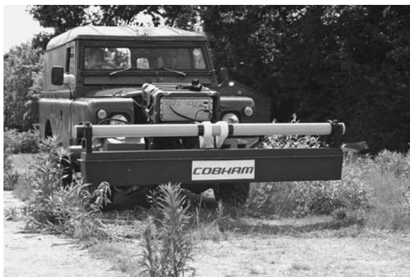
FIGURE 7.15 Eight channel GPR system on trials on Land Rover (with kind permission ©ERA Technology).
