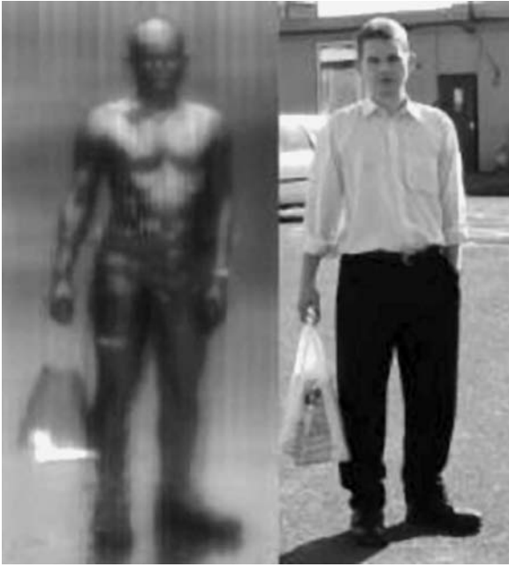
FIGURE 7.20 A 94-GHz system millimeter-wave image taken outdoors with visual image for comparison (with kind permission QinetiQ).
